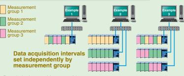
By assigning input modules to one of three measurement groups, you can set measuring intervals for signals from transients to temperature on a group-by-group basis.
