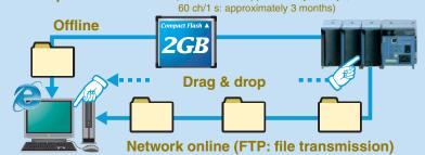
Point a Web browser to URL of the MW100 to send MW100 data files with drag-and-drop ease
