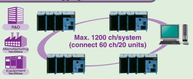
With MXLOGGER (sold separately), you can quickly set up a large-scale data acquisition system of up to 1200 ch/20 units with no programming required.
